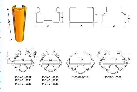
\* iFlex RackGuards are also available in 400mm,1000mm and bespoke sizes, as well as with internal rubber lugs.
